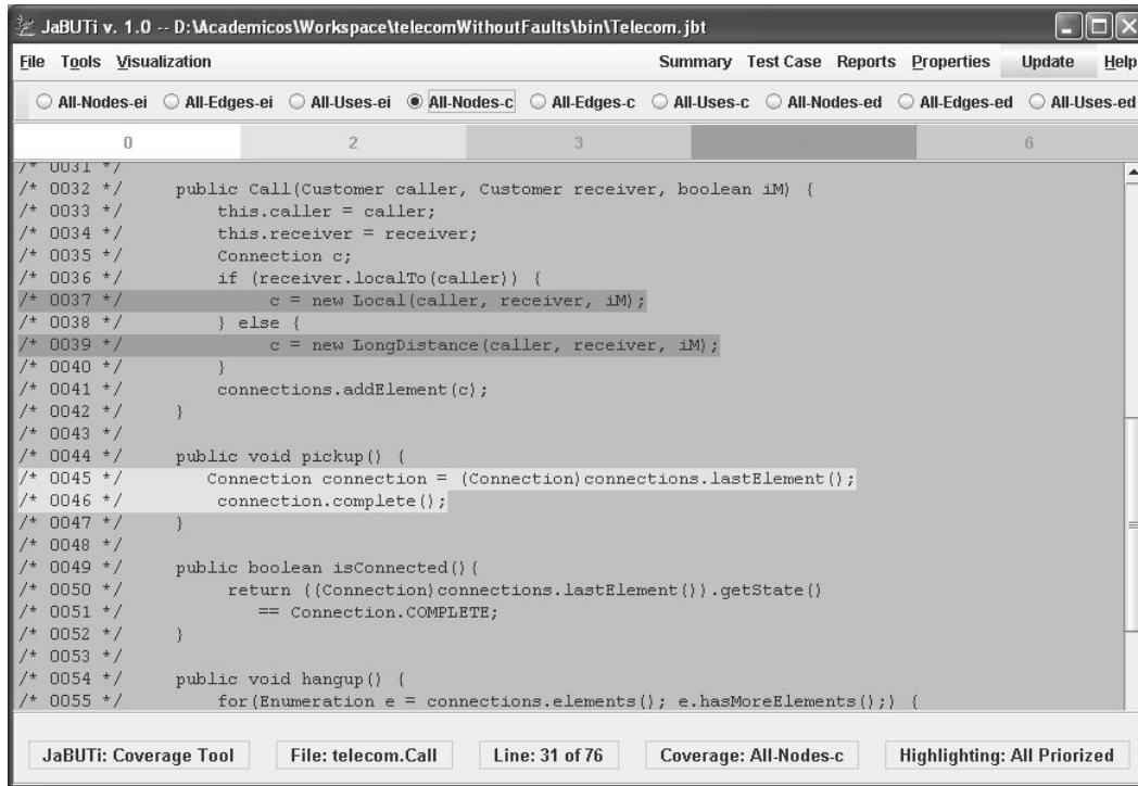
Fig. 11. Part of the source code of the Call class with the all-crosscutting-nodes testing requirements highlighted.
